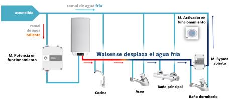
When hot water is going to be used, the WAISENSE Activator is triggered to start the recirculation of the system. During this process the Power Module drives the cold water in the hot water pipes to the Bypass Module, where it is returned to the circuit, without the need for additional pipes or water tanks. As soon as the water reaches the desired temperature, the Bypass Module stops the recirculation and the Activator signals the end of recirculation.
